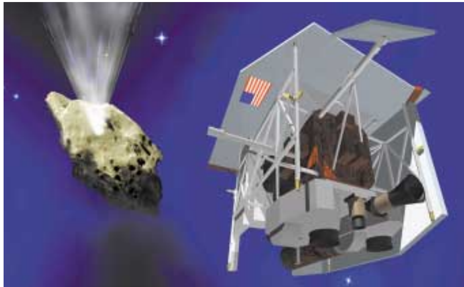
NASA'S DEEP IMPACT MISSION, which will project a 500 kilogramme solid impactor into a comet, Temple 1 (artist's impression). A flyby spacecraft will take images and make measurements. The impactor will also take images of the comet's surface prior to impact. The mission aims to increase understanding of the composition and structure of comets.
