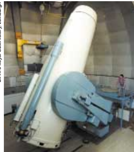
THE 1.2 METRE UNITED KINGDOM SCHMIDT TELESCOPE at the Anglo-Australian Observatory, Siding Spring, Australia has conducted many all-sky surveys since the mid-1990s. The resulting plate archive at Edinburgh is proving very valuable in determining asteroid orbits. The telescope was used specifically for an asteroid survey between 1990 and 1992 in a programme led by Dr Duncan Steel.
